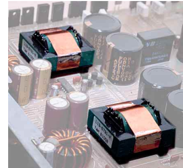
Dual power supply means the final stage of amplification won't rob power from the driver stage, which can cause distortion in single-supply car amps when demand is heavy.
